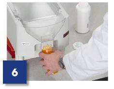
**Fill Vial** - Use vial to lift funnel gate and allow pills to flow into vial.
